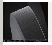
Roughened lens edge, effectively prevents glare induced by the lens edge.
